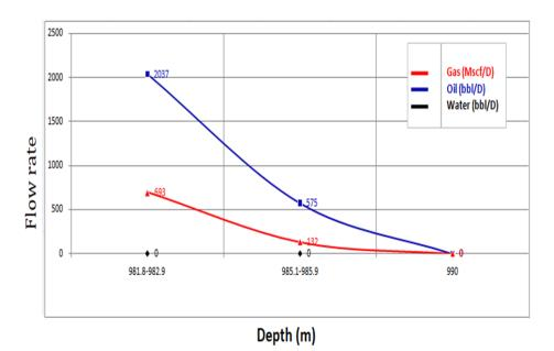
Figure 5. Third flowing by choke 64/64"
