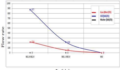
Depth (m) Figure 3. First flowing using choke 32/64"
