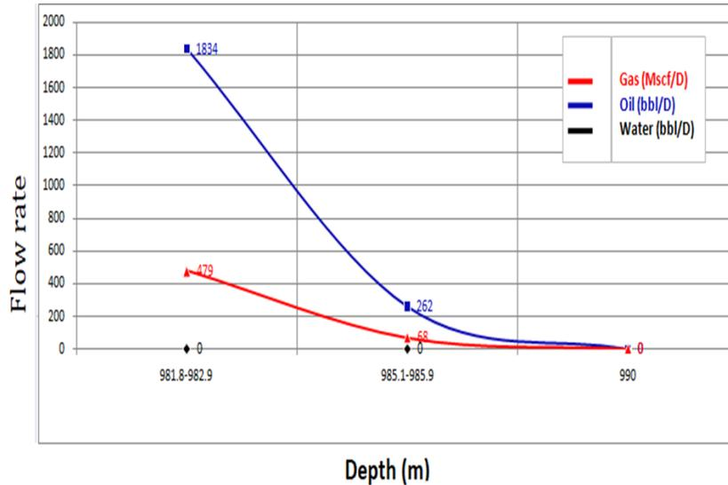
Figure 4. Second flowing by choke 48/64"
