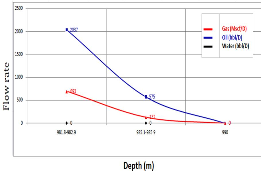
Figure 5. Third flowing by choke 64/64"
