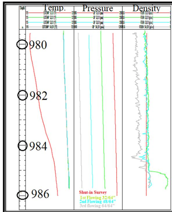
Figure 2. Density, temperature, and pressure comparison of all survey
