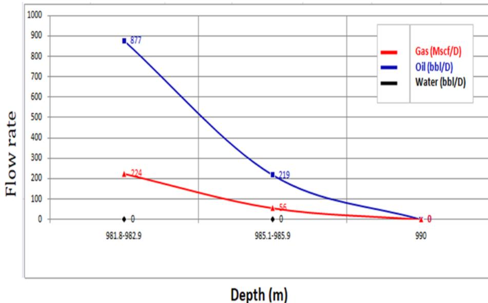
**Figure 3.** First flowing using choke 32/64"
