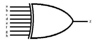
Figure 2: the XOR gate with eight inputs
