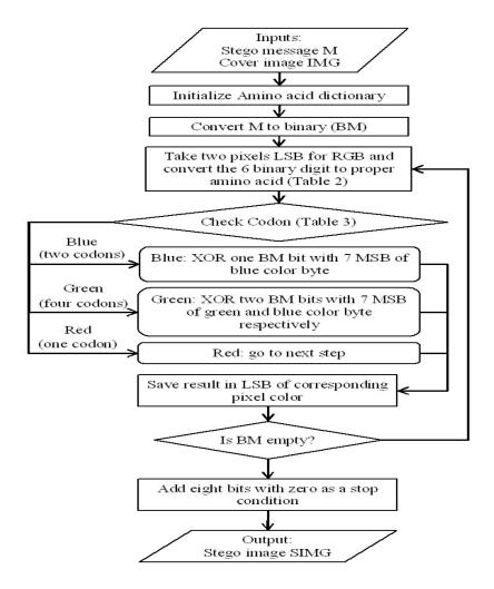
Figure 1: Data hiding phase flow chart
