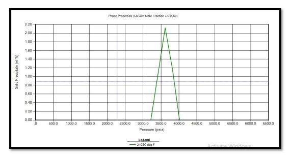
Figure 2. Asphaltene precipitation curve for well A
