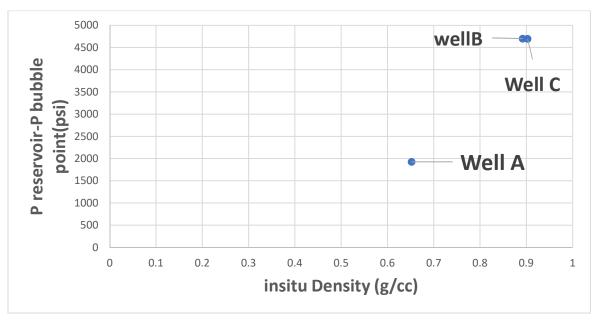
Figure 6. A remade version of the De Boer plot showing the three wells
