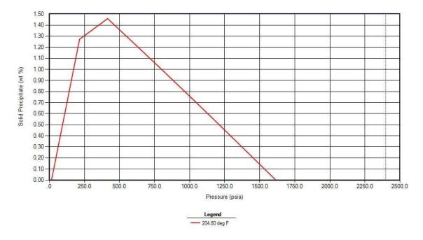
Figure 4. Asphaltene precipitation curve for well C
