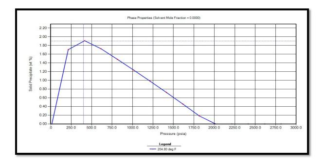
Figure 3. Asphaltene precipitation curve for well B
