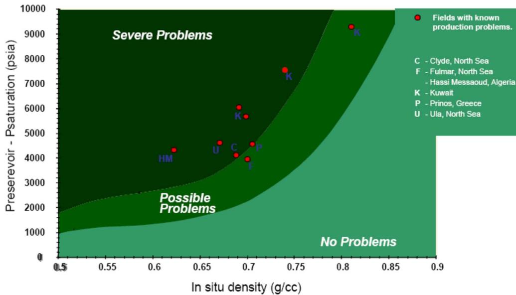
Figure 5. De Boers' plot for asphaltene problem prediction (De Boer et al., 1995)
