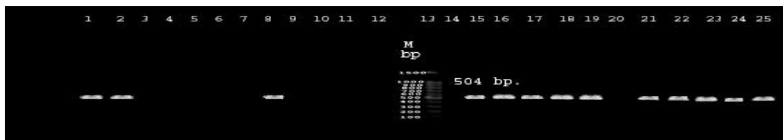
Figure 4. PCR amplification of the exoS gene with a molecular weight of 504 bp following electrophoresis on a 1.5% agarose gel that was run at 5 V/cm for 2 hours. Line M contained the DNA molecular weight marker (1,500–100bp)
