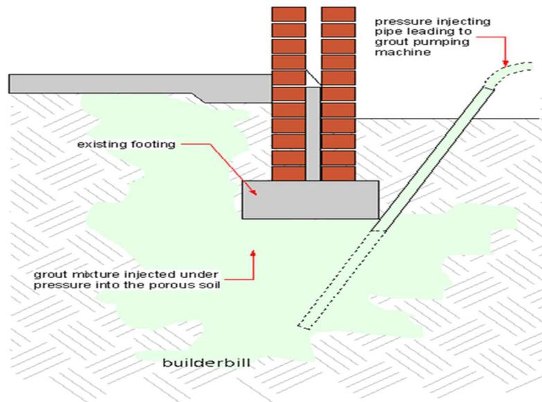
Figure 9. Underpinning - Injecting a grout mixture into the sub soil under the weak foundation (Ghiassi et al., 2011)
