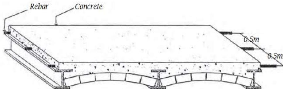
Figure 7. Typical detail of increasing rigidity of the ceilings (Afshari, 2017)
