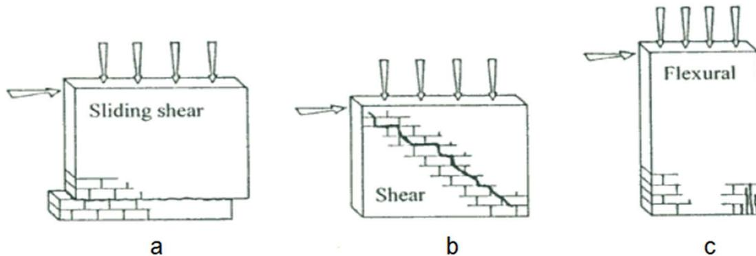
Figure 1. Typical failure modes of unreinforced masonry walls, subjected to in-plane loads: (a) Sliding Shear failure, (b) Shear failure, and (c) Flexural failure (Garbin et al., 2007)
