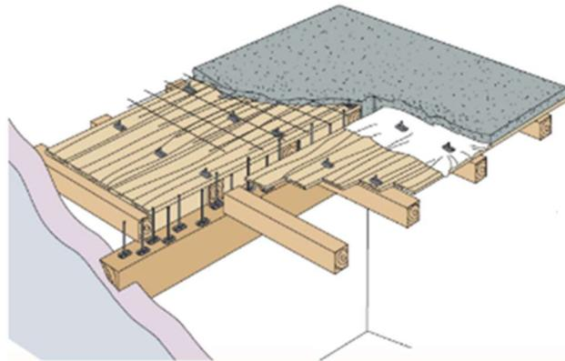
Figure 6. The reducing wooden ceilings weight with a cooperating reinforced concrete slab (Meireles et al., 2013)
