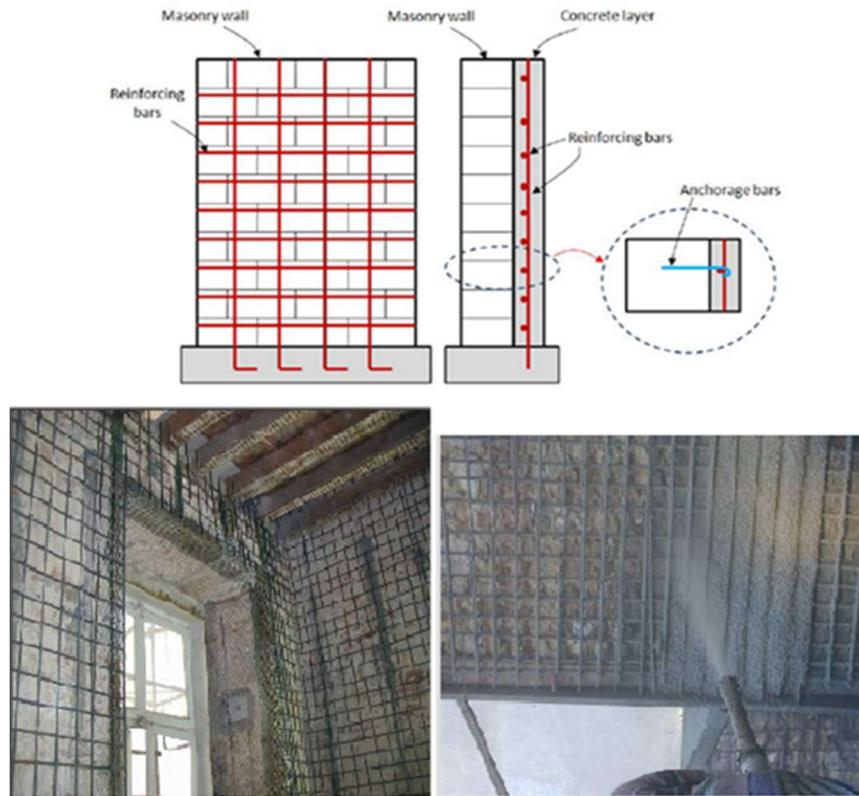
Figure 2. Typical detail of masonry wall strengthening with reinforced concrete layer (Ghiassi et al., 2011; Meireles et al., 2013)
