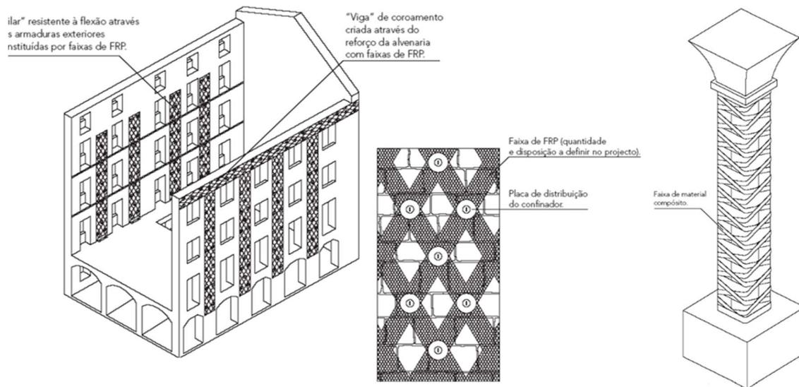
Figure 4. Application of CFRP/GFRP on building, wall and column (Meireles et al., 2013)
