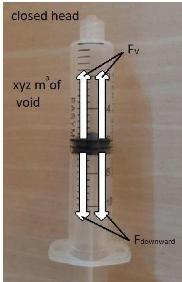
**Figure 1.** The void creation experiment setup with the use of a closed head syringe
