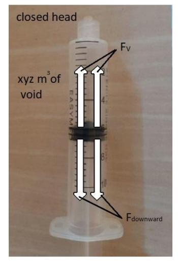
Figure 1. The void creation experiment setup with the use of a closed head syringe
