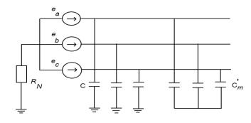
Figure 3. Conversion of the capacitive conductance of the power line
