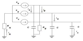
Figure 1. Equivalent circuit for an overhead transmission line with a single phase-ground fault
