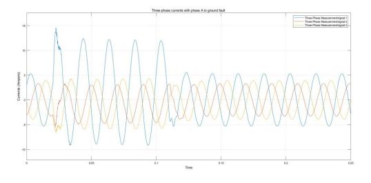
Figure 11. Three-phase current when a phase A-to-ground fault occurs with connecting C, Rn, and Rg.
