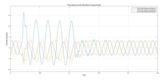
Figure 10. Three-phase current when a phase A-to-ground fault occurs with connecting C and Rn but without connecting Rg.
