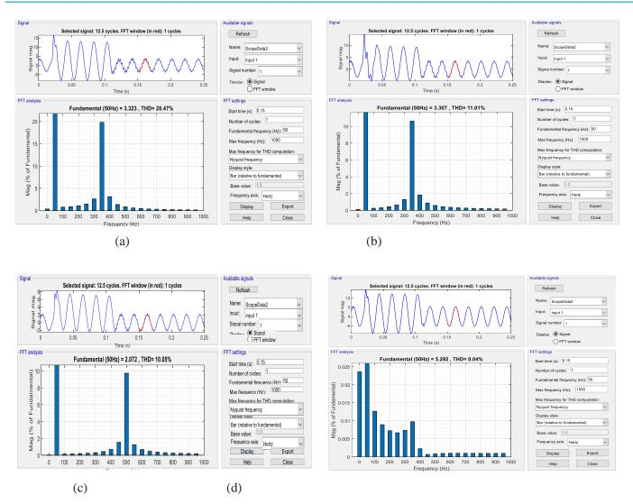
Figure 12. Harmonic analysis of phase current A when a phase A-to-ground fault occur (**a**) without connecting C,  $R_n$ , and  $R_g$ , (**b**) when connecting C, but  $R_n$  and  $R_g$  are not connected, (**c**) when connecting C and  $R_n$ , but  $R_g$  is not connected, and (**d**) when connecting C,  $R_n$ , and  $R_g$
