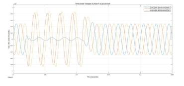
Figure 7. Three-phase voltages with occurrence of a phase A to ground fault
