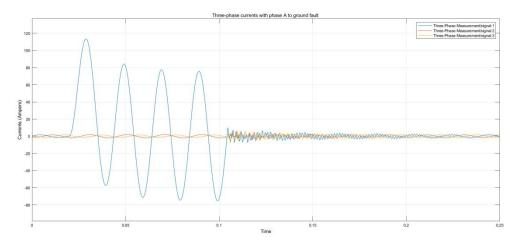
Figure 8. Three-phase current when a phase A-to-ground fault occurs without connecting C, Rn, and Rg.
