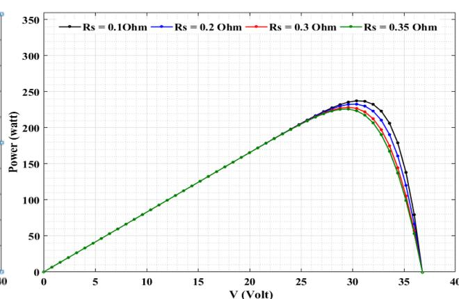
Figure 7. The P-V characteristics of the PV module with different series resistance.
