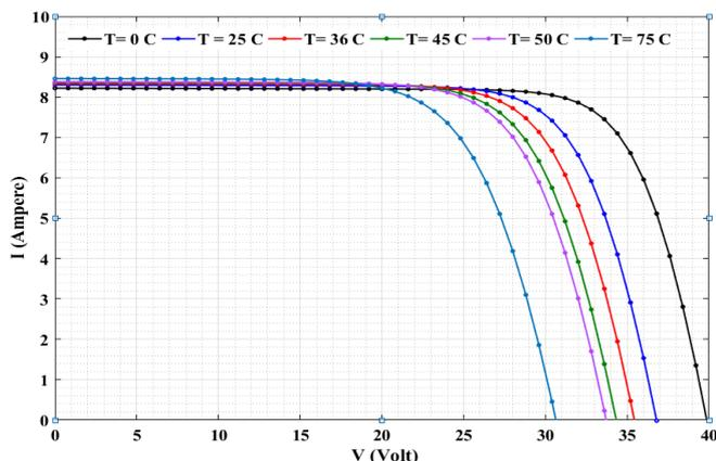
Figure 4. The I-V characteristics of the PV module with different temperatures.
