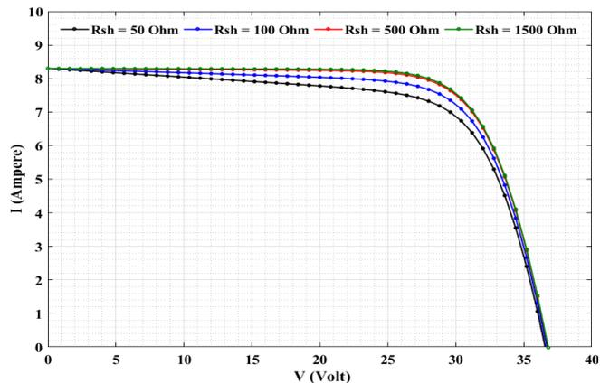
Figure 8. The I-V characteristics of the PV module with different shunt resistance.
