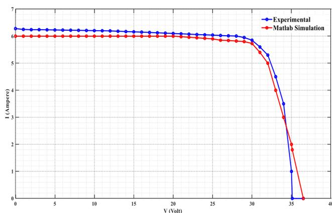
Figure 13. The I-V characteristics for both the practical experimental and Matlab simulations.
