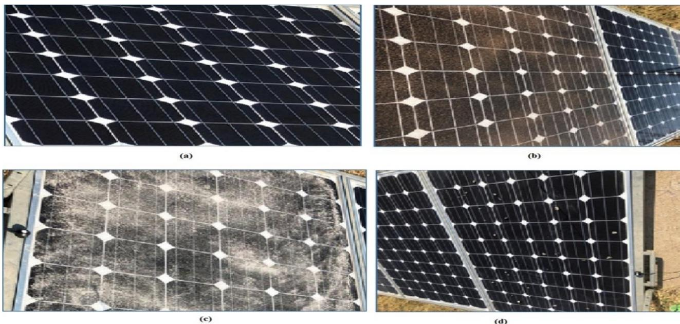
Figure 12. Actual photos for the present PV system with the different environmental states: (a) The reference case (clean PV Panel), (b) dust collection, (c) chalk powder, (d) bird droppings.
