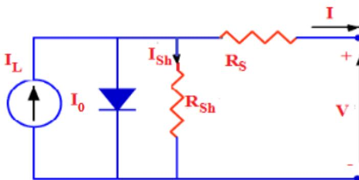
Figure 1. The schematic diagram of a single diode solar cell.
