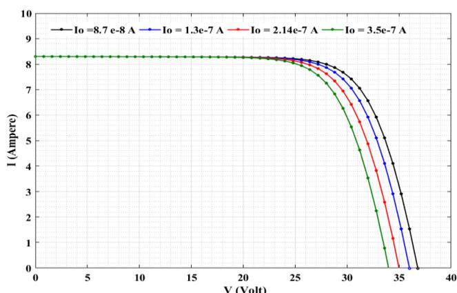
Figure 10. The effect of saturation current on I-V characteristics.
