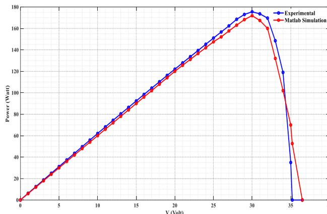
Figure 14. The P-V characteristics for both practical experimental and Matlab simulations.
