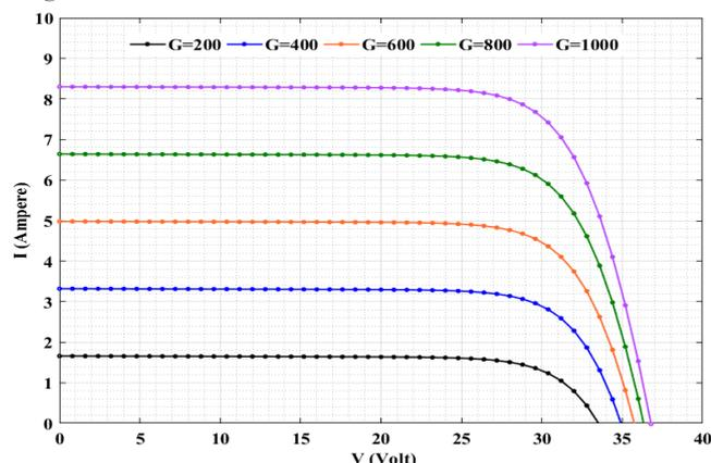
Figure 2. The I-V characteristics for different solar radiation.
