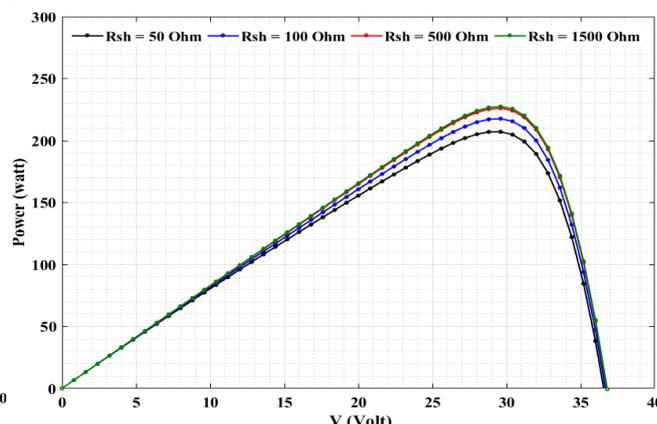
Figure 9. The P-V characteristics of the PV module with different shunt resistance.
