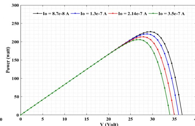
Figure 11. The effect of saturation current on P-V characteristics.
