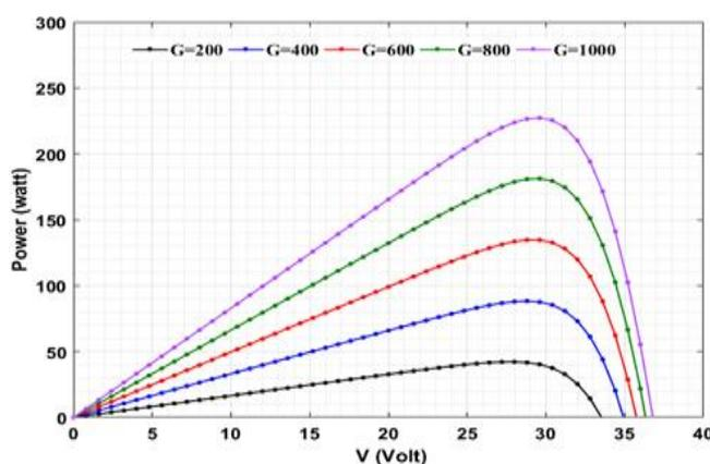
Figure 3. The P-V characteristics for different solar radiation.
