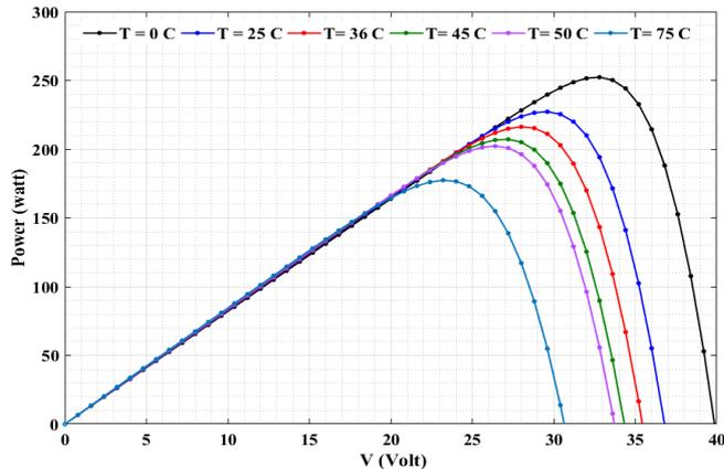
Figure 5. The P-V characteristics of the PV module with different temperatures.
