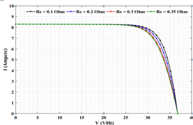
Figure 6. The I-V characteristics of the PV module with different series resistance.
