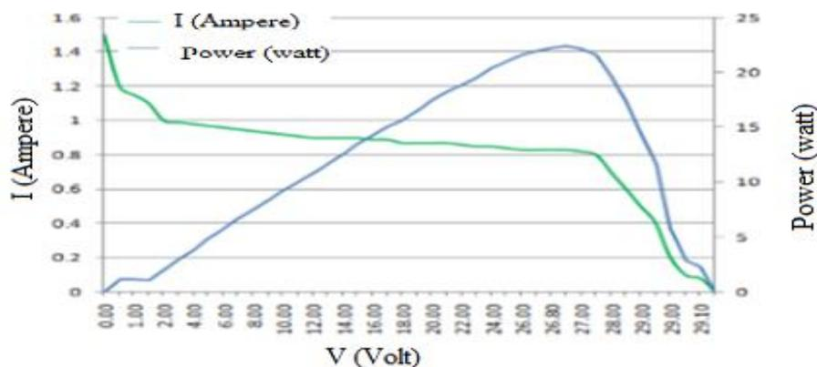
Figure 15. The I-V and P-V characteristics for solar panels exposed to cloudy weather - Erbil City.
