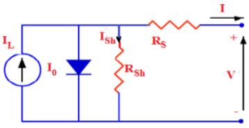
Figure 1. The schematic diagram of a single diode solar cell.
