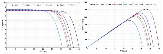
Figure 4. The I-V characteristics of the PV module with Figure 5. The P-V characteristics of the PV module with different temperatures.
