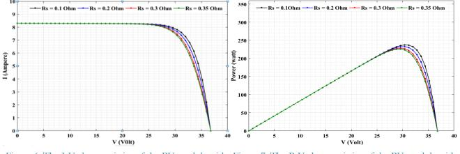
Figure 6. The I-V characteristics of the PV module with Figure 7. The P-V characteristics of the PV module with different series resistance.
