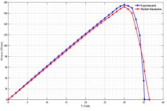
Figure 14. The P-V characteristics for both practical experimental and Matlab simulations.
