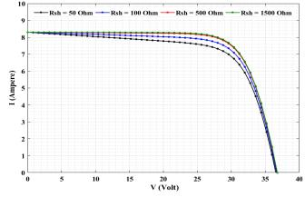
Figure 8. The I-V characteristics of the PV module with Figure 9. The P-V characteristics of the PV module with different shunt resistance.
