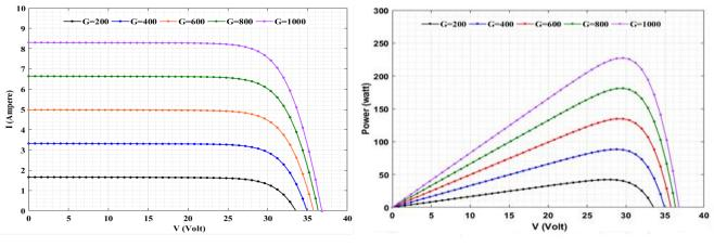
Figure 2. The I-V characteristics for different solar radiation.
