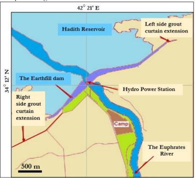
Figure 5. An illustrative map showing the length of Haditha Dam, the earthfill left and right banks, and left and right side grout curtain extensions (Adamo et al., 2018b). The authors added approximate scale and coordinates.
