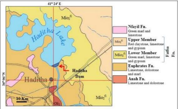
Figure 3. Geological map of Haditha Dam site and reservoir area (From Sissakian et al., 2018).
