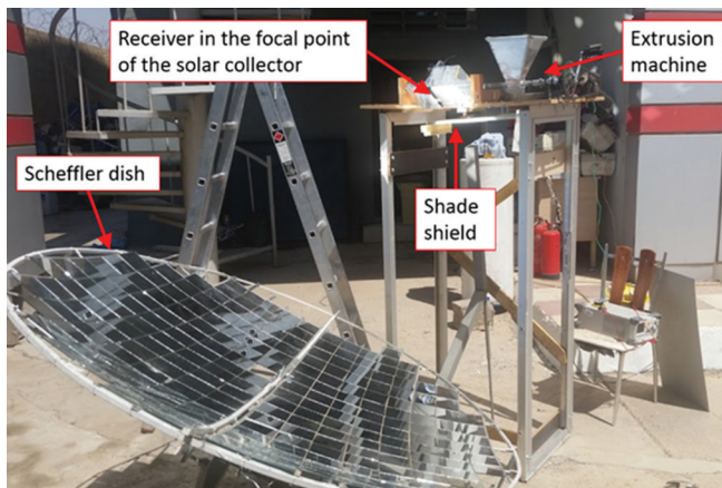
Figure 2. The extrusion machine is mounted on a stand, so the receiver is in the focal point of the solar collector
