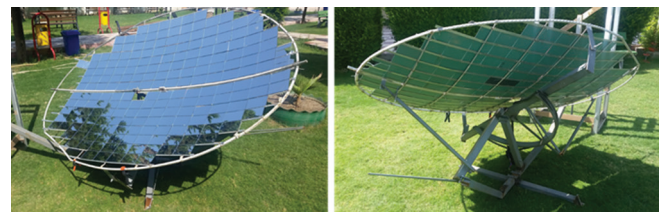
Figure 1. Scheffler solar collector created for this work
