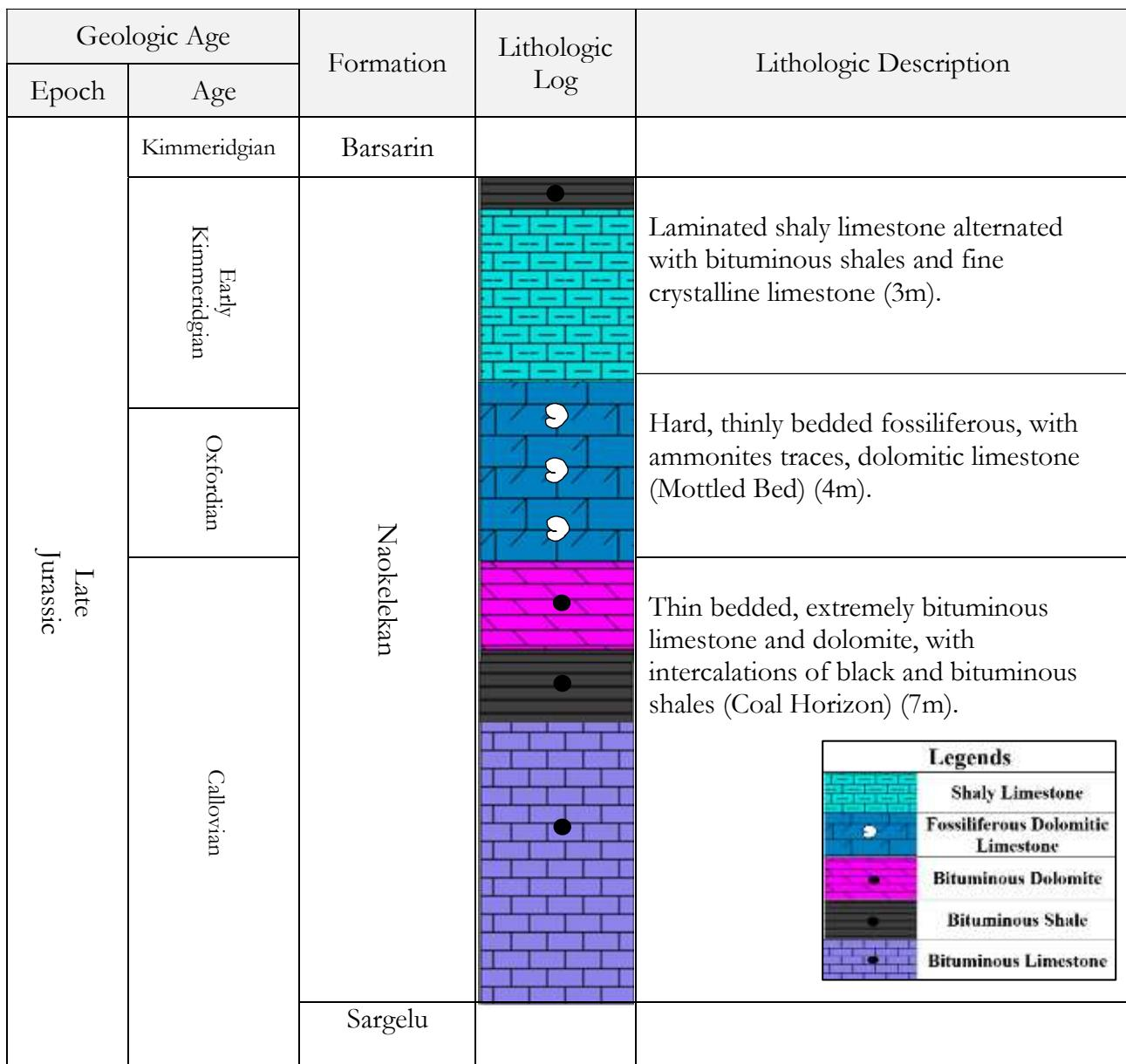
Figure 2. A Stratigraphic column manifesting the first formal description of Naokelekan Formation in its type section at Naokelekan Village, Erbil. (outlined from Morton and Wetzel 1950 in Bellen *et al.*, 1959). No vertical Scale. The whole section is 14 m.
