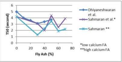
Figure 4. Effect of fly ash content on slump flow time (T50).
