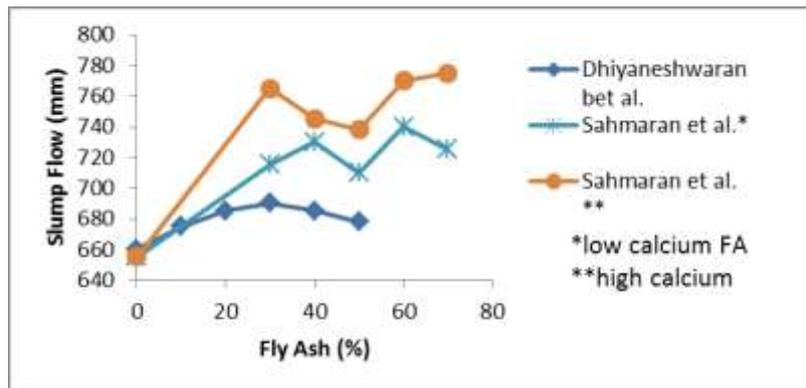
Figure 3. Effect of fly ash content on slump flow.
