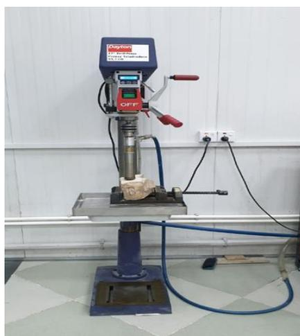
Figure 2c. Drill Press (core plugging machine).
