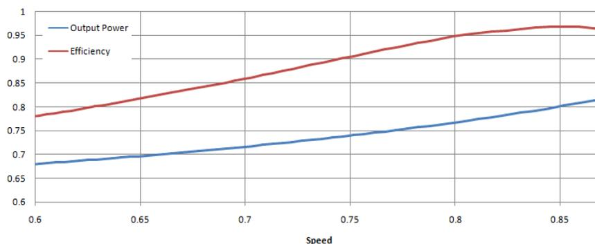
Figure 5. Efficiency and output-power vs. speed curves.
