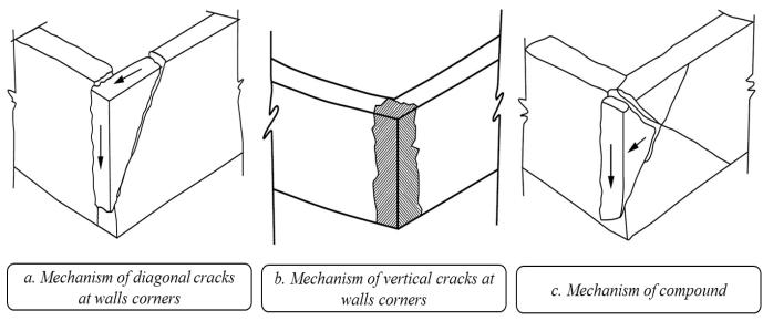
Figure 4. Mechanism of Cracks at Corners (Mardani et al., 2019).
