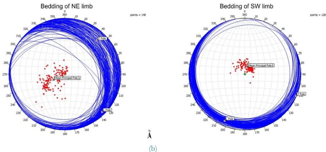
Figure 5. (a) Stereograms showing density contours for fracture poles. Red colours represent high density, (b) Lower hemisphere equal area stereograms for bedding planes.
