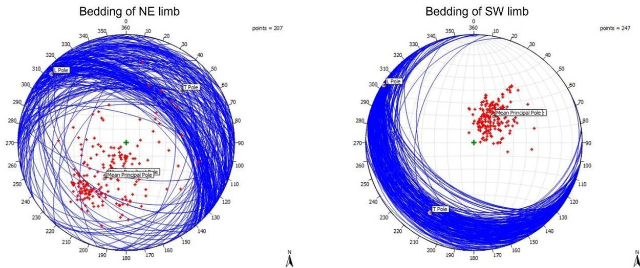
Figure 3. (a) Stereograms showing density contours for fracture poles. Red colours represent high density, (b) Lower hemisphere equal area stereograms for bedding planes. Bedding planes plotted as great circles in blue and poles to bedding planes in red.
