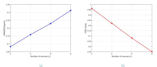
Figure 13. The impact of the number of sources on DoA estimation accuracy. (a) ARMSE vs. number of sources, (b) PSD (DoA) vs. number of sources.
