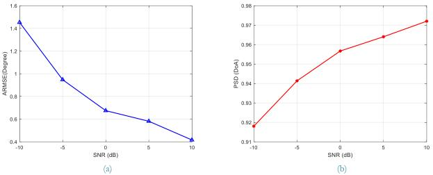
Figure 3. The Impact of SNR variations on DoA estimation performance. (a) ARMSE vs. SNR, (b) PSD (DoA) vs. SNR.
