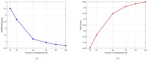
Figure 5. The Impact of number of snapshots on DoA estimation performance. (a) ARMSE vs. Number of snapshots, (b) PSD(DoA) vs. Number of snapshots.
