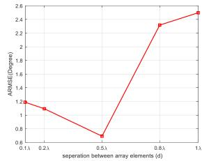
Figure 11. Illustration of optimum inter-element spacing of the array in terms of estimation error.
