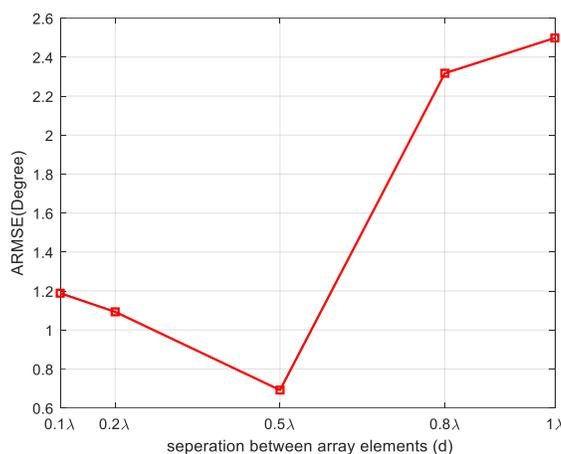
Figure 11. Illustration of optimum inter-element spacing of the array in terms of estimation error.
