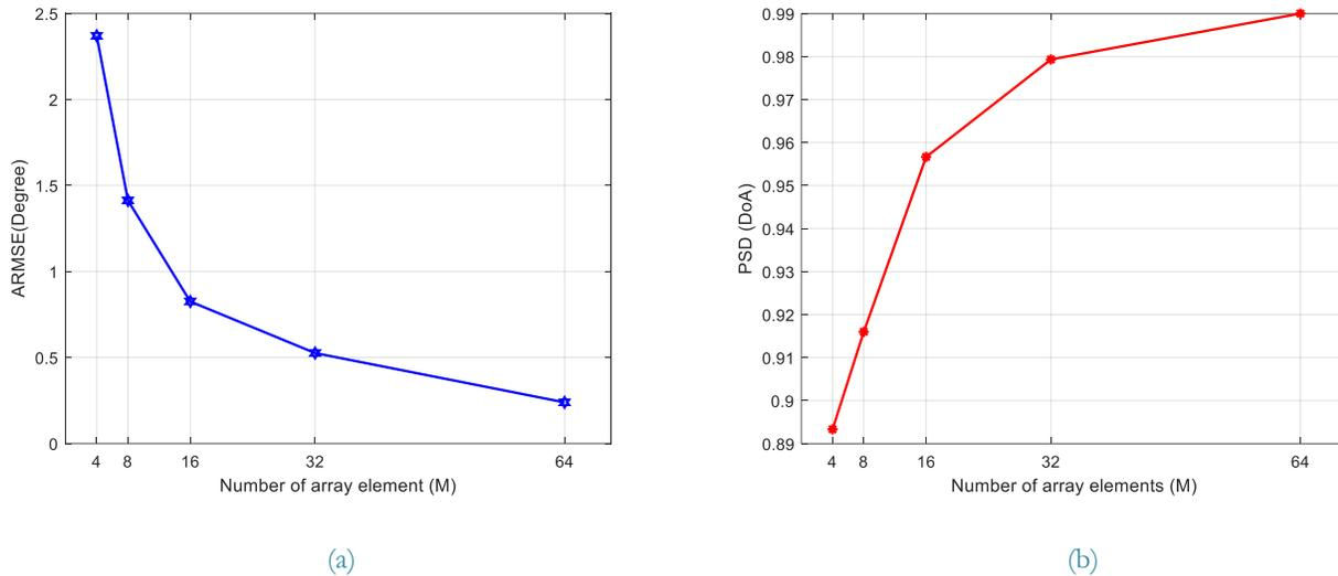
Figure 8. The Impact of number of array elements on DoA estimation performance. (a) ARMSE vs. Number of array elements, (b) PSD(DoA) vs. Number of array elements.
