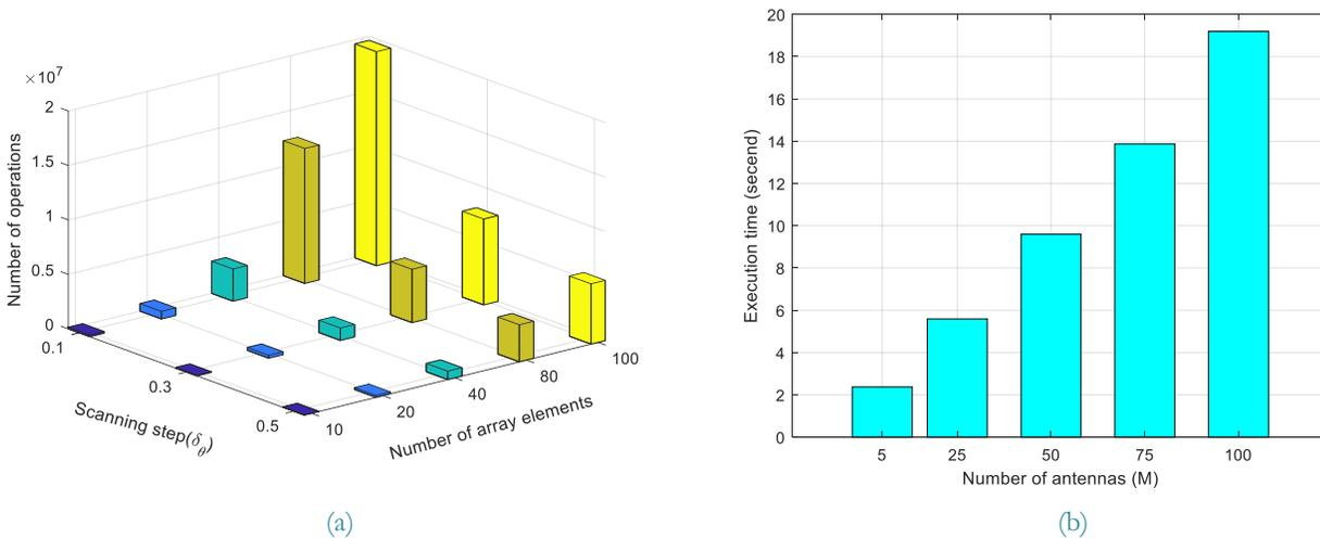
Figure 9. The impact of array size on DoA estimation complexity. (a) overall computational complexity vs array elements and different scanning steps, (b) execution time (second) vs number of array elements.
