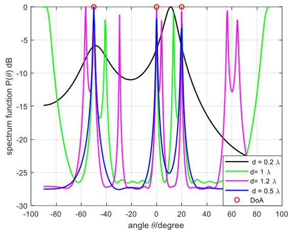
Figure 10. The impact of spatial separation between array elements on estimation resolution.
