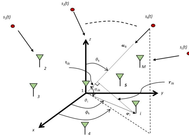
Figure 1. DoA problem formulation with  $M$ -element arbitrary array and  $L$  sources.
