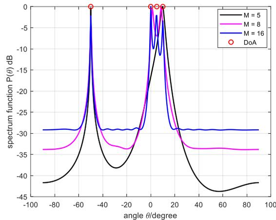
Figure 7. The impact of the number of array elements on DoA estimation resolution.
