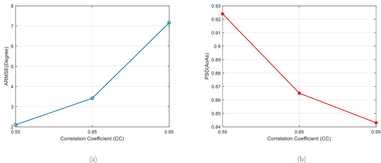
Figure 15. the impact of correlated sources on DoA estimation performance. (a) ARMSE vs. CC, (b) PSD(DoA) vs. CC.
