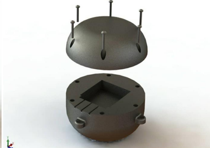
Figure 6. Open view of shielding ECU design.
