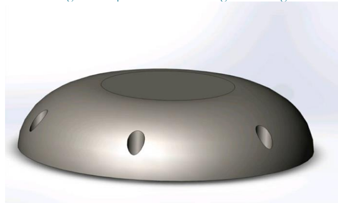
Figure 8. Top view of the shielding ECU design (ECU solid cover).
