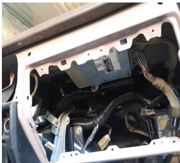
Figure 3. Installation location of Toyota Tactical Vehicle ECU 4.5F.
