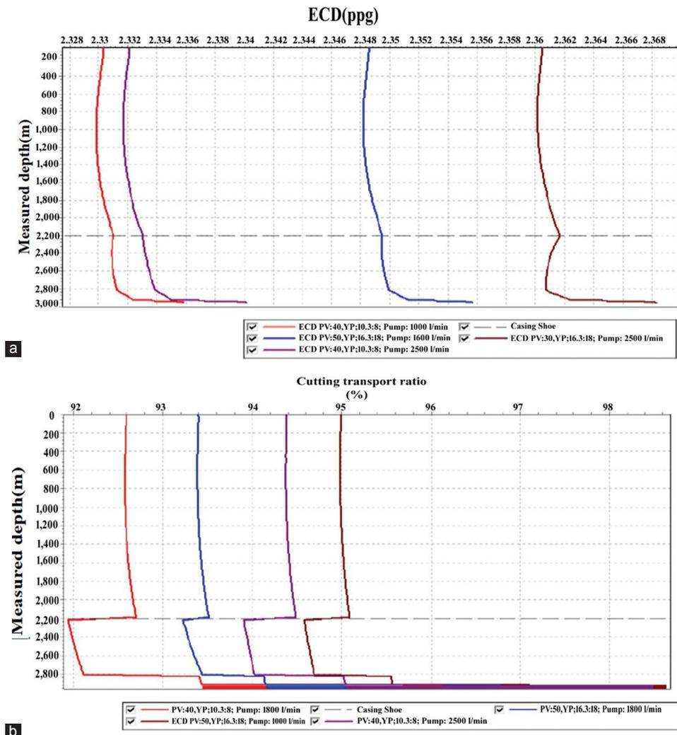
Figure 6. (a) ECD measured depth relationship, (b) cutting transport ratio and measured depth relationship for MW=2.30 gm/cm³
