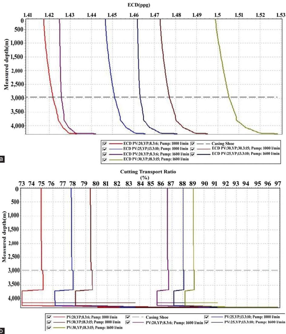
Figure 7. (a) ECD measured depth relationship, (b) cutting transport ratio and measured depth relationship for MW=1.35 gm/cm<sup>3</sup>
