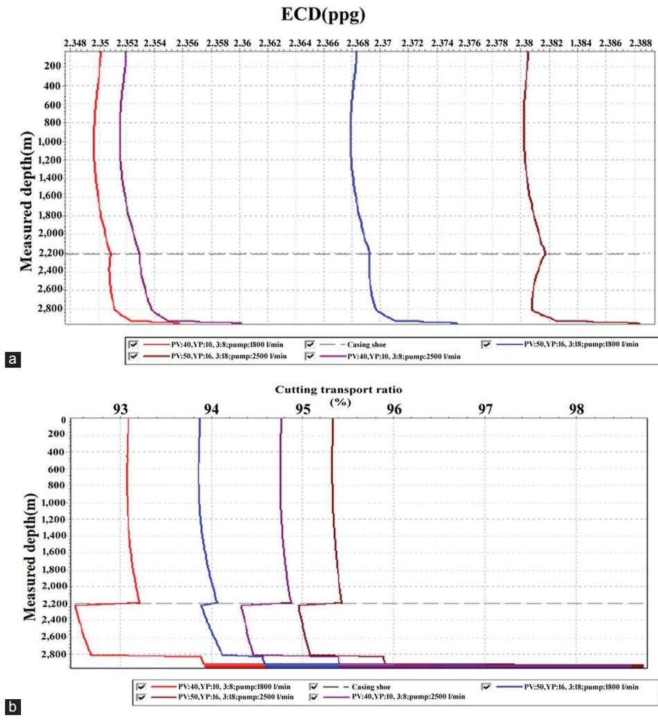
Figure 5. (a) ECD measured depth relationship, (b) cutting transport ratio and measured depth relationship for MW=2.32 gm/cm<sup>3</sup>
