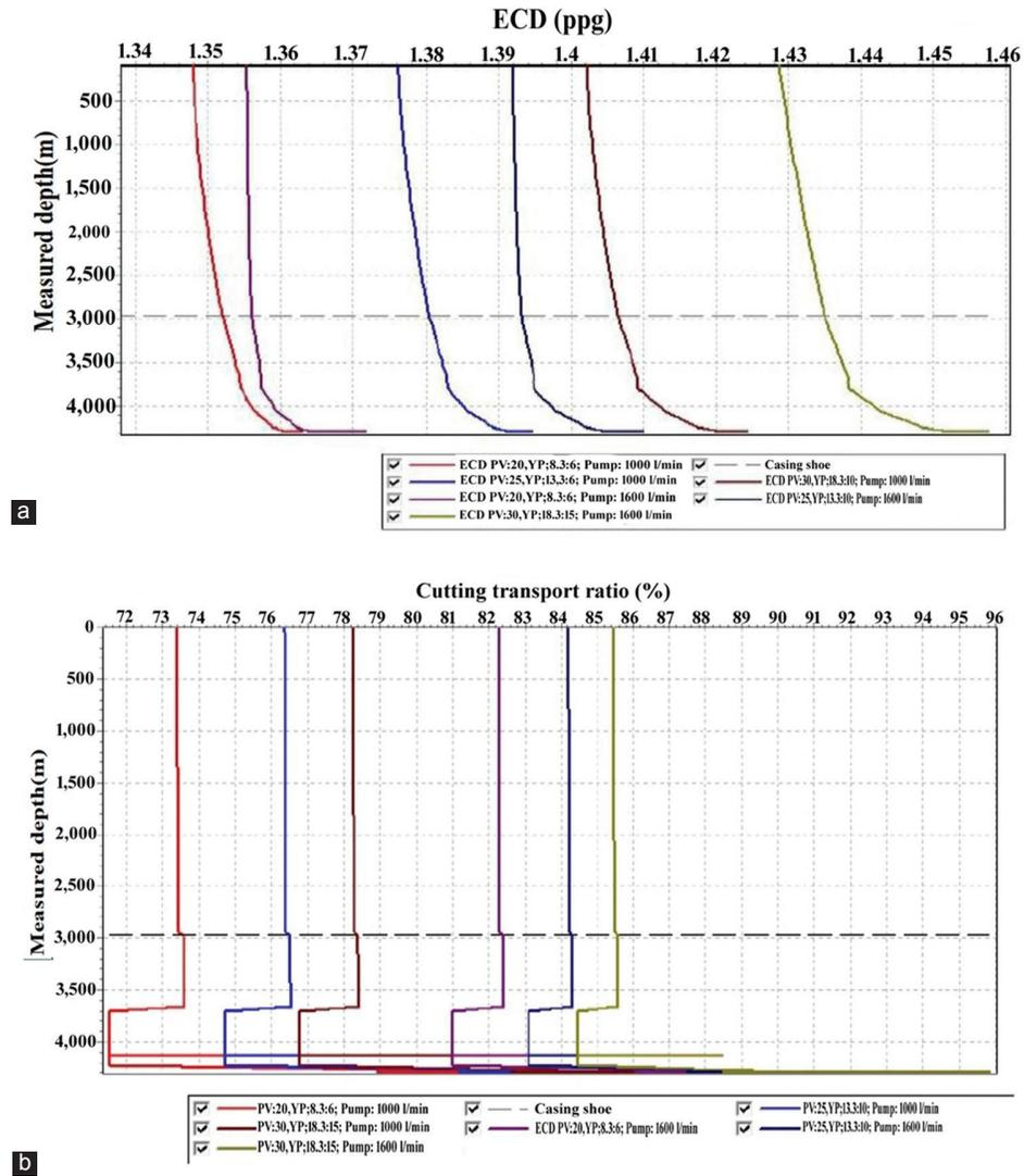
Figure 4. (a) ECD measured depth relationship, (b) cutting transport ratio and measured depth relationship for MW=1.36 gm/cm<sup>3</sup>
