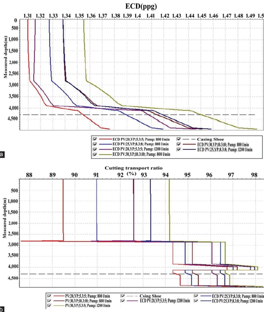
Figure 9. (a) ECD measured depth relationship, (b) cutting transport ratio and measured depth relationship for MW=1.26 gm/cm<sup>3</sup>
