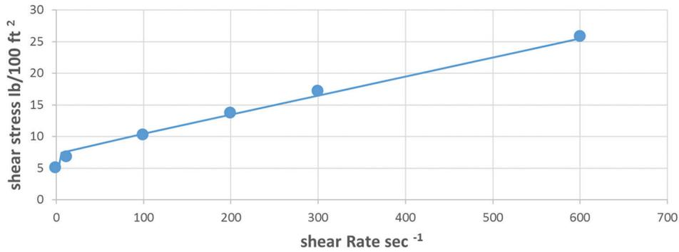
Figure 1. Shear rate and shear stress relationship
