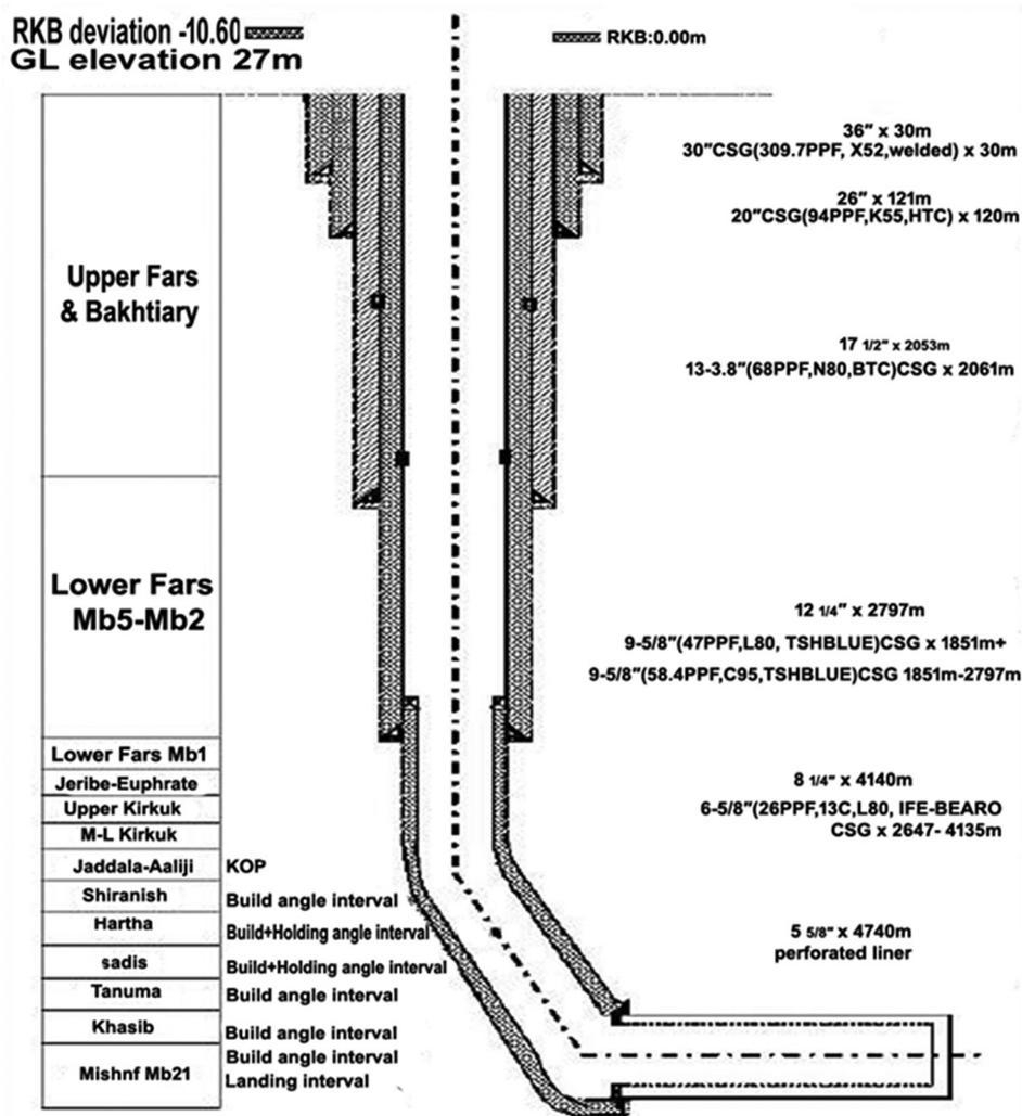
Figure 2. Schematic of the horizontal well
