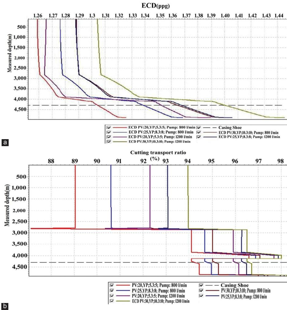
Figure 8. (a) ECD measured depth relationship, (b) cutting transport ratio and measured depth relationship for MW=1.21 gm/cm<sup>3</sup>
