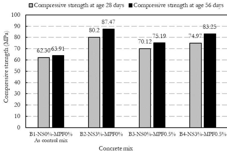
Figure 11. Compressive strength of concrete mix at age 28 and 56 days.
