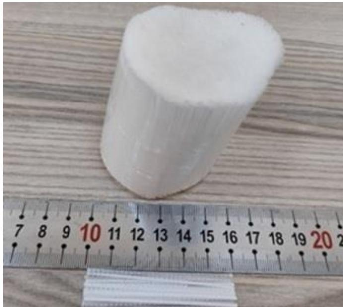
Figure 6. Shape of Macro-type polypropylene fiber.
