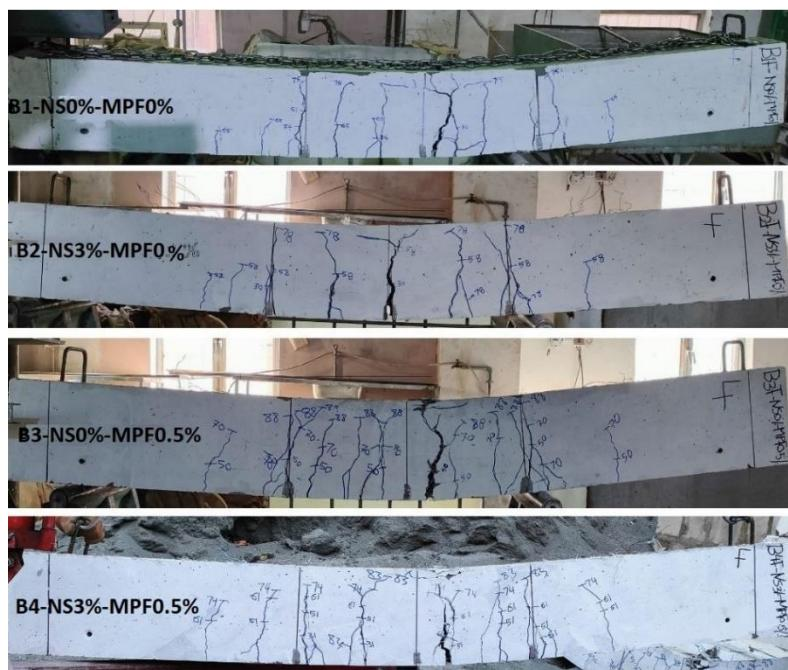
Figure 17. Crack patterns of tested beams.
