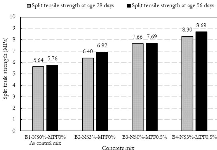
Figure 12. Indirect tensile strength of concrete mix at age 28 and 56 days.
