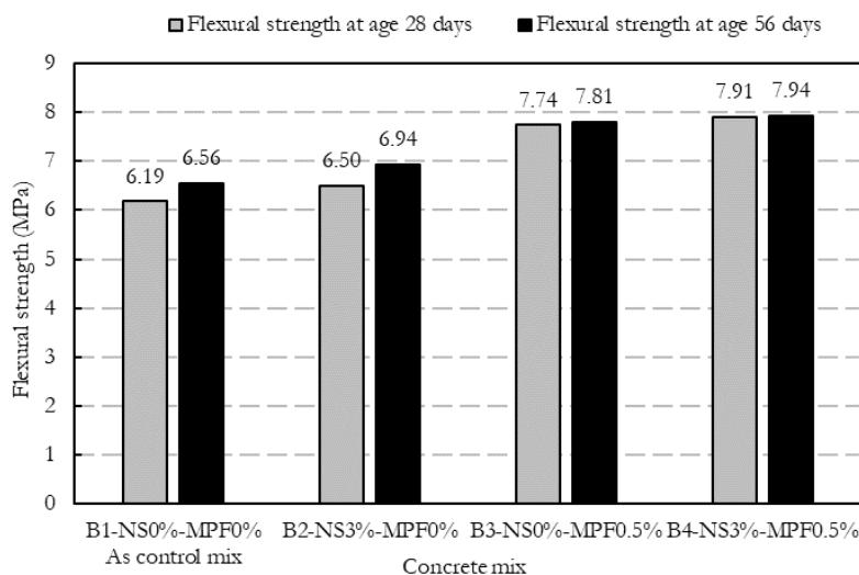
Figure 13. Flexural strength of concrete mix at age 28 and 56 days.
