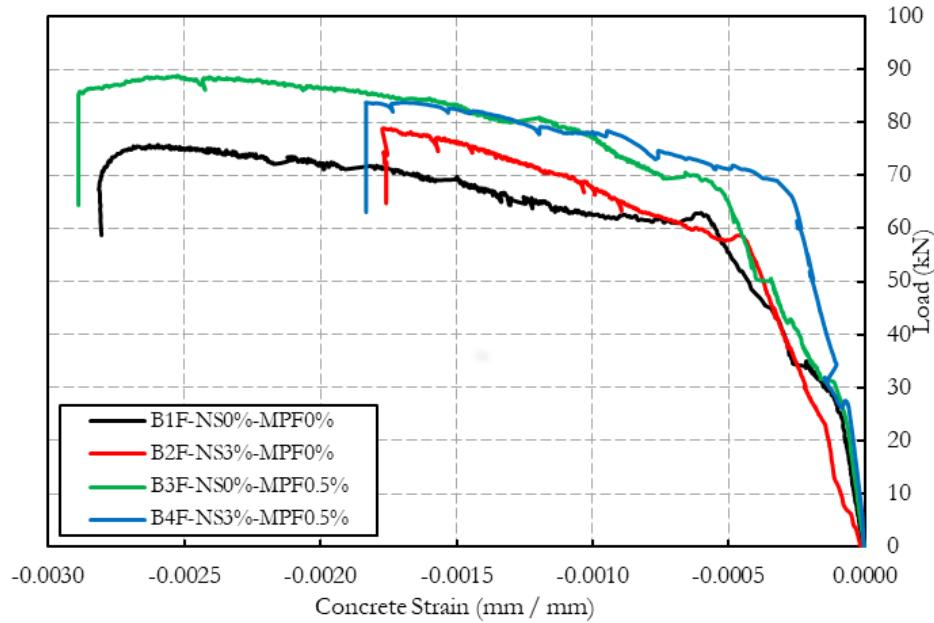
Figure 15. Load – Concrete compressive strain.
