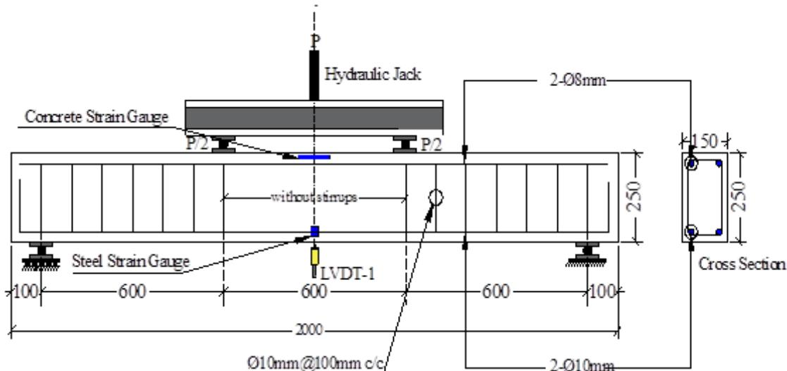
Figure 8. Details of test beams.
