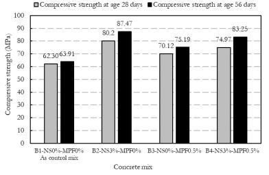
Figure 11. Compressive strength of concrete mix at age 28 and 56 days.
