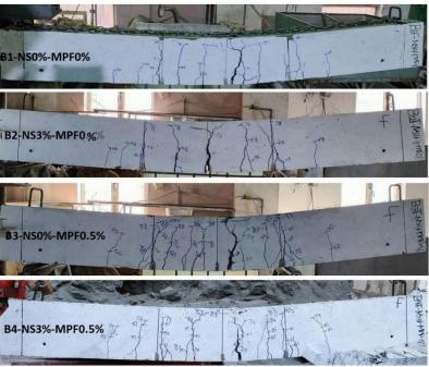
Figure 17. Crack patterns of tested beams.
