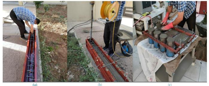
Figure 9. a) Formwork molds, b) Casting of beam specimens, and c) Vibration table of cylinders and prisms.
