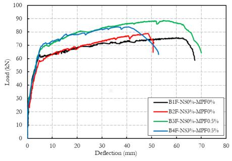
Figure 14. Load-mid span deflection relationship for all mixes.
