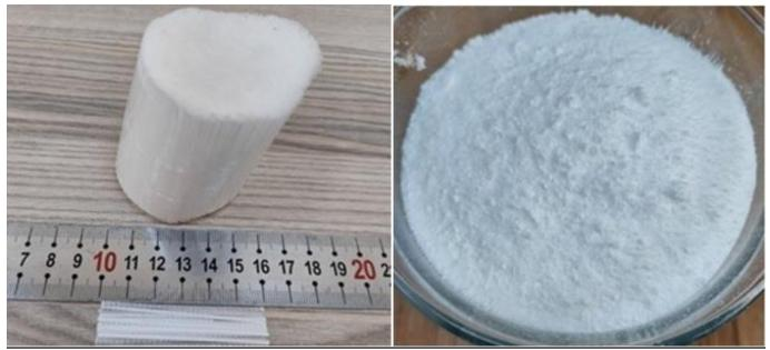
Figure 6. Shape of Macro-type polypropylene fiber.
