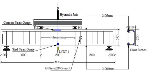
Figure 8. Details of test beams.
