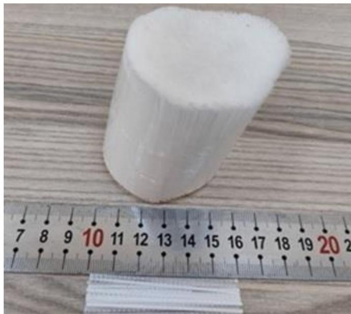
*Figure 6. Shape of Macro-type polypropylene fiber.*
