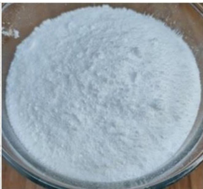
*Figure 7. Appearance of powdery Nano-silica.*
