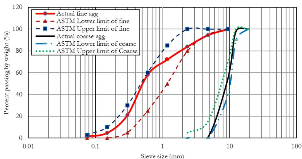
Figure 5. Aggregate gradation curve with ASTM C33 standard limits for fine and coarse aggregates.
