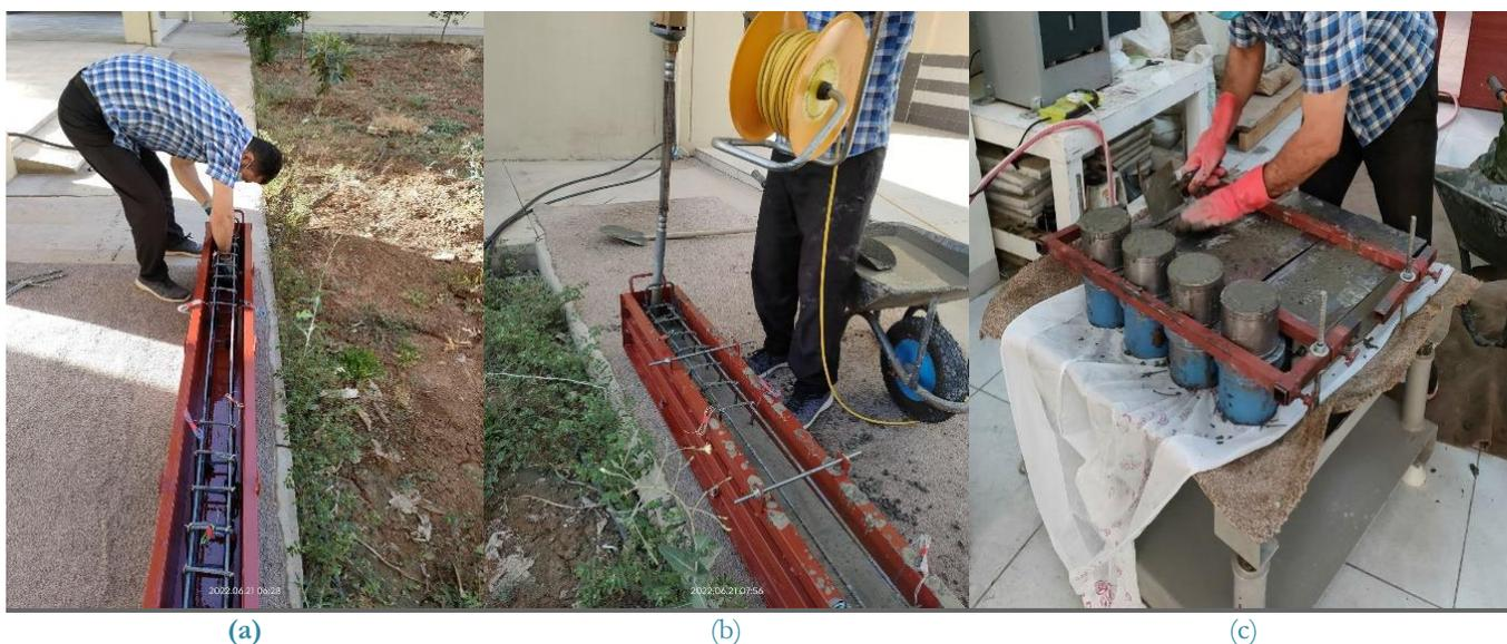
Figure 9. a) Formwork molds, b) Casting of beam specimens, and c) Vibration table of cylinders and prisms.
