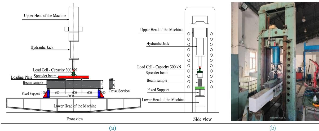
Figure 10. a) Schematic presentation of loading frame, and b) Beam test loading frame instrument.
