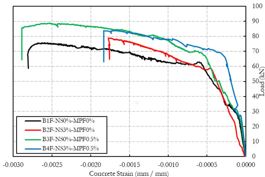
Figure 15. Load – Concrete compressive strain.
