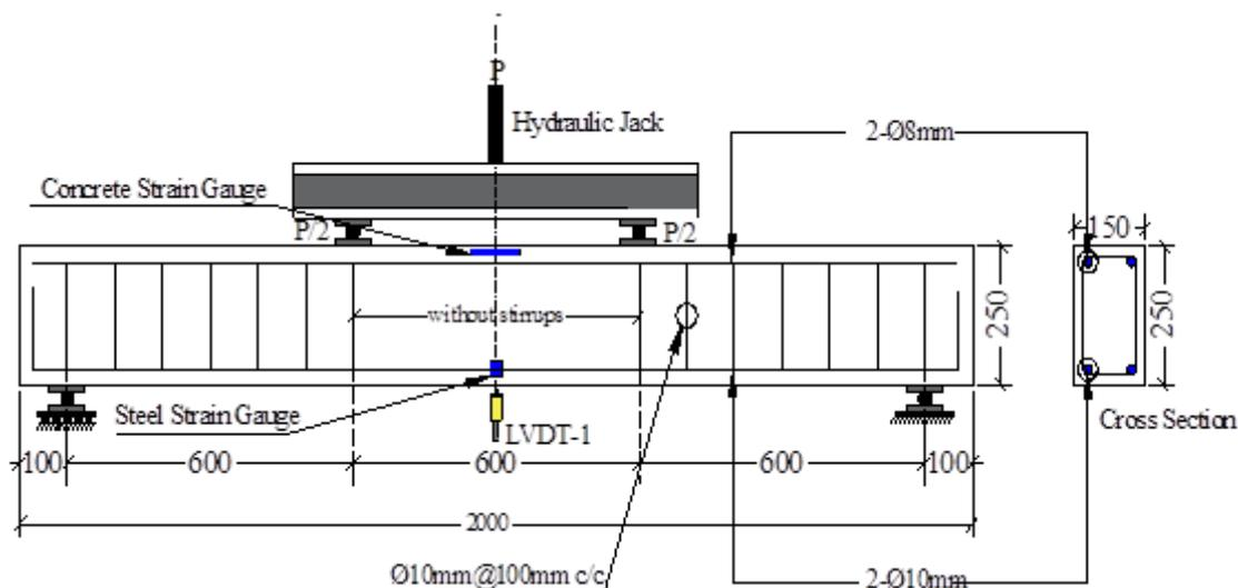
Figure 8. Details of test beams.
