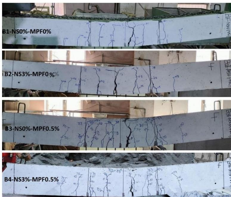
Figure 17. Crack patterns of tested beams.
