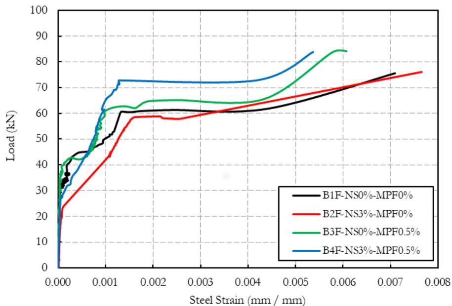
Figure 16. Load – Bottom steel strain.
