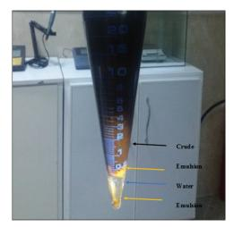
Figure 9. Crude separation with heterogeneous mixture
