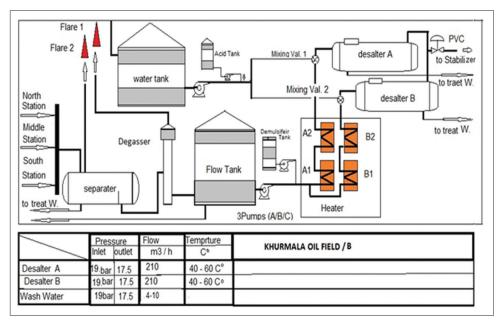
Figure 7. Process flow diagram of desalting process at Khurmala oil field with acid injection
