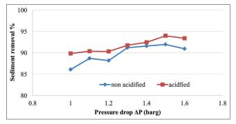
Figure 22. Effect of pressure drop on sediment removal
