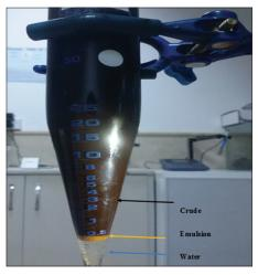
Figure 8. Crude separation phases
