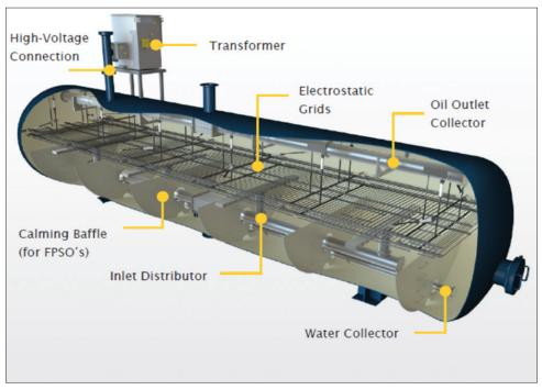
Figure 3. Desalter electrostatic coalescence process (Group, 2017)
