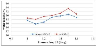
Figure 23. Effect of pressure drop on water removal
