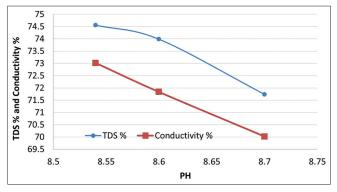
Figure 14. Relation between total dissolved solids, conductivity, and pH at basic condition
