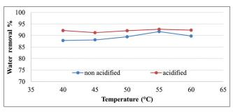
Figure 20. Effect of temperature on water removal
