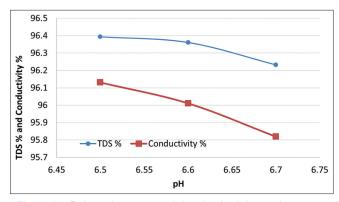
Figure 15. Relation between total dissolved solids, conductivity, and pH at acid condition
