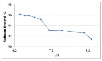
Figure 17. Desalter efficiency in acidic condition with sediment removal
