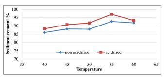
Figure 18. Effect of temperature on sediment removal
