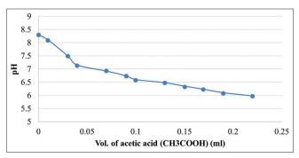
Figure 13. Volume of acetic acid required for reducing the pH of wash water
