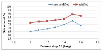
Figure 21. Effect of pressure drop on salt removal
