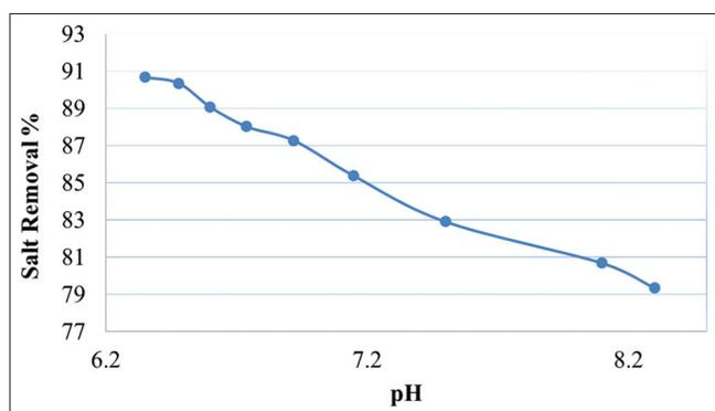
Figure 16. Desalter efficiency with salt removal
