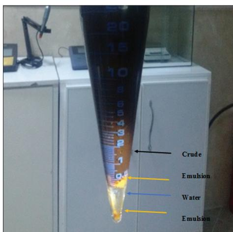
Figure 9. Crude separation with heterogeneous mixture
