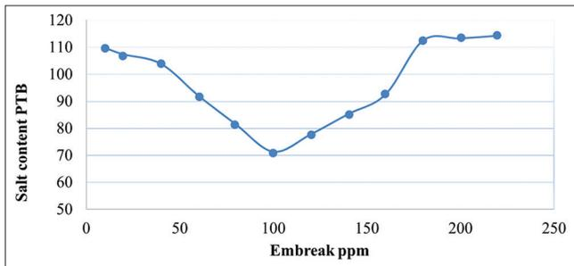
Figure 11. Behavior of salt content with dosage
