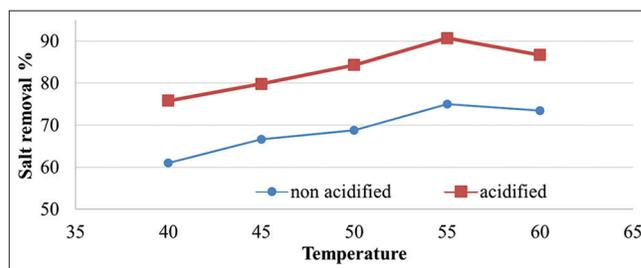
Figure 19. Effect of temperature on salt removal
