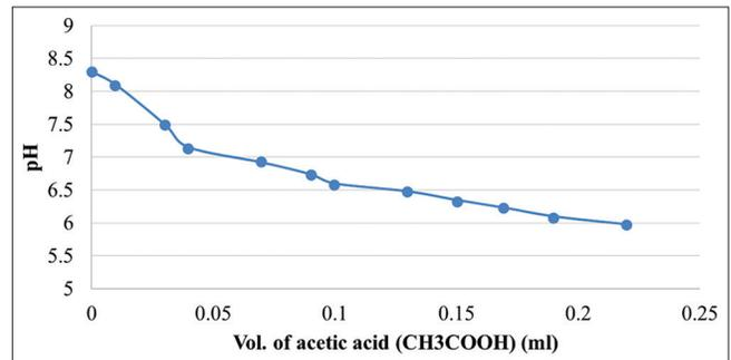
Figure 13. Volume of acetic acid required for reducing the pH of wash water
