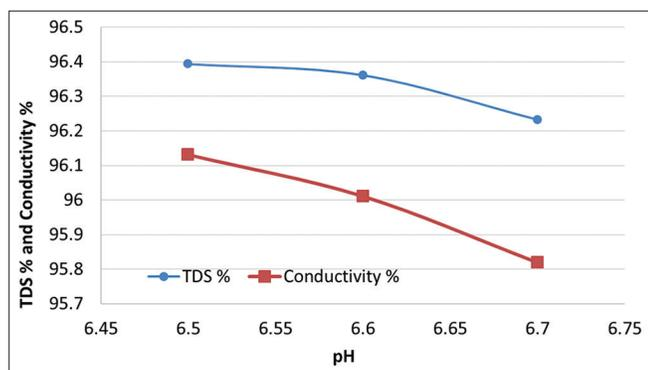
Figure 15. Relation between total dissolved solids, conductivity, and pH at acid condition
