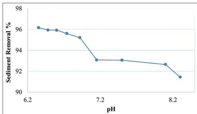
Figure 17. Desalter efficiency in acidic condition with sediment removal
