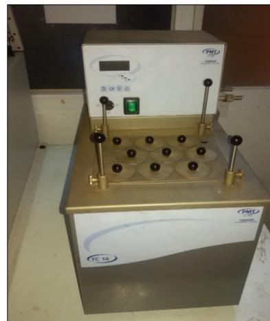
Figure 4. Bath water temperature (PM Tamson Inst.)
