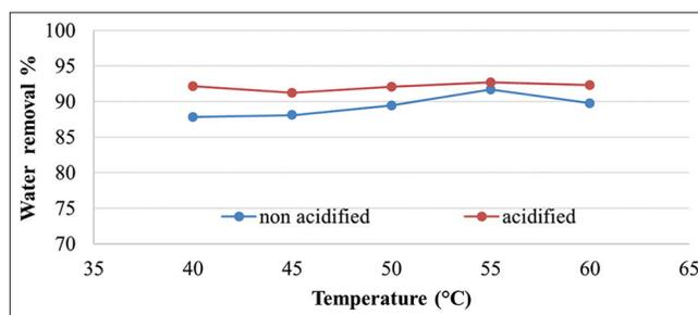
Figure 20. Effect of temperature on water removal
