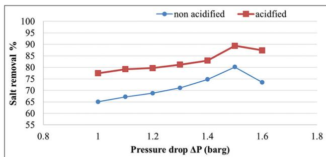
Figure 21. Effect of pressure drop on salt removal
