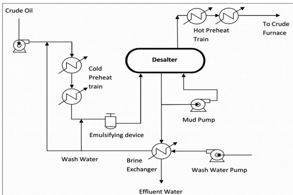
Figure 2. Complete flow system of the desalting process (Mason *et al.*, 1995)
