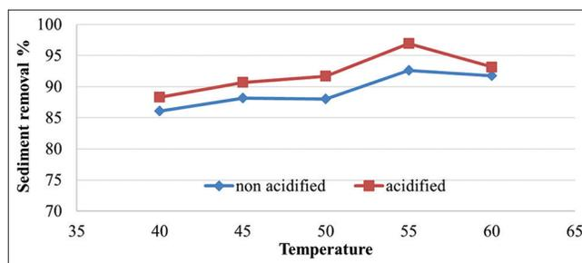
Figure 18. Effect of temperature on sediment removal
