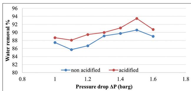
Figure 23. Effect of pressure drop on water removal
