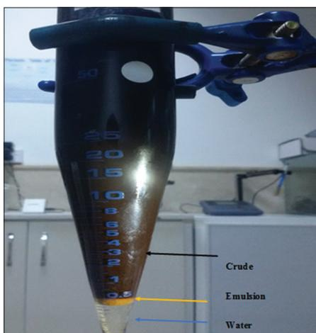
Figure 8. Crude separation phases
