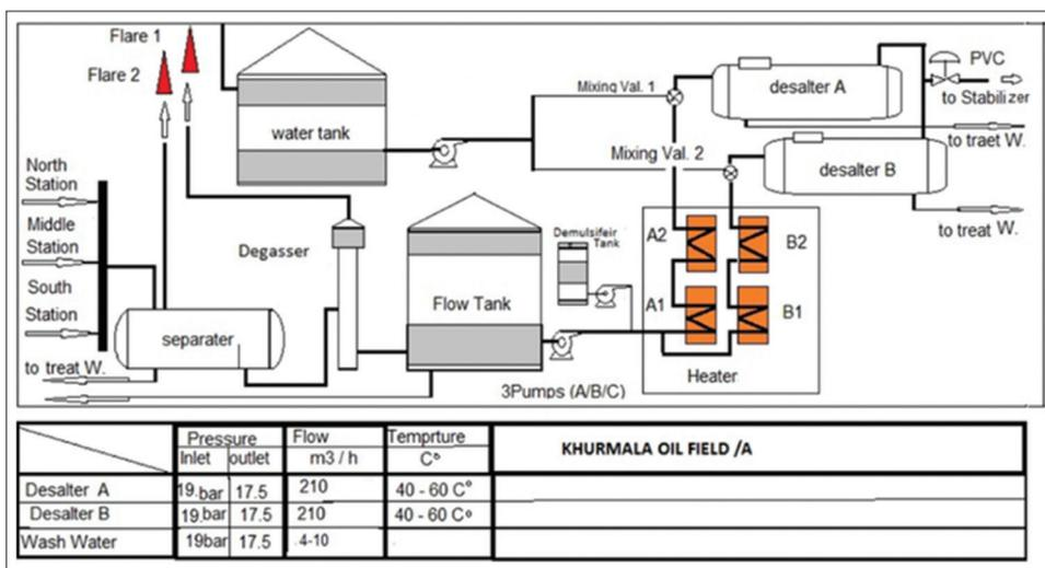
Figure 6. Process flow diagram of desalting process at Khurmala oil field without acid injection
