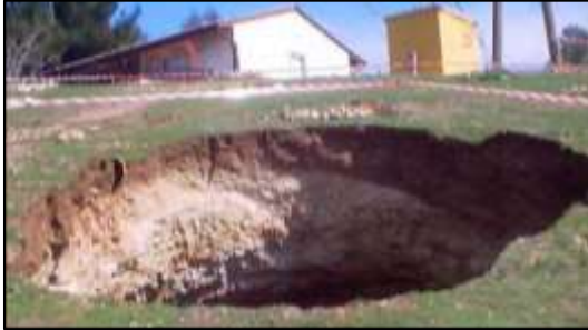
Figure 3. A Recent Developed Sinkhole (Down-Stream) After Filling of the Reservoir (Al-Ansari et al. , 2015b).
